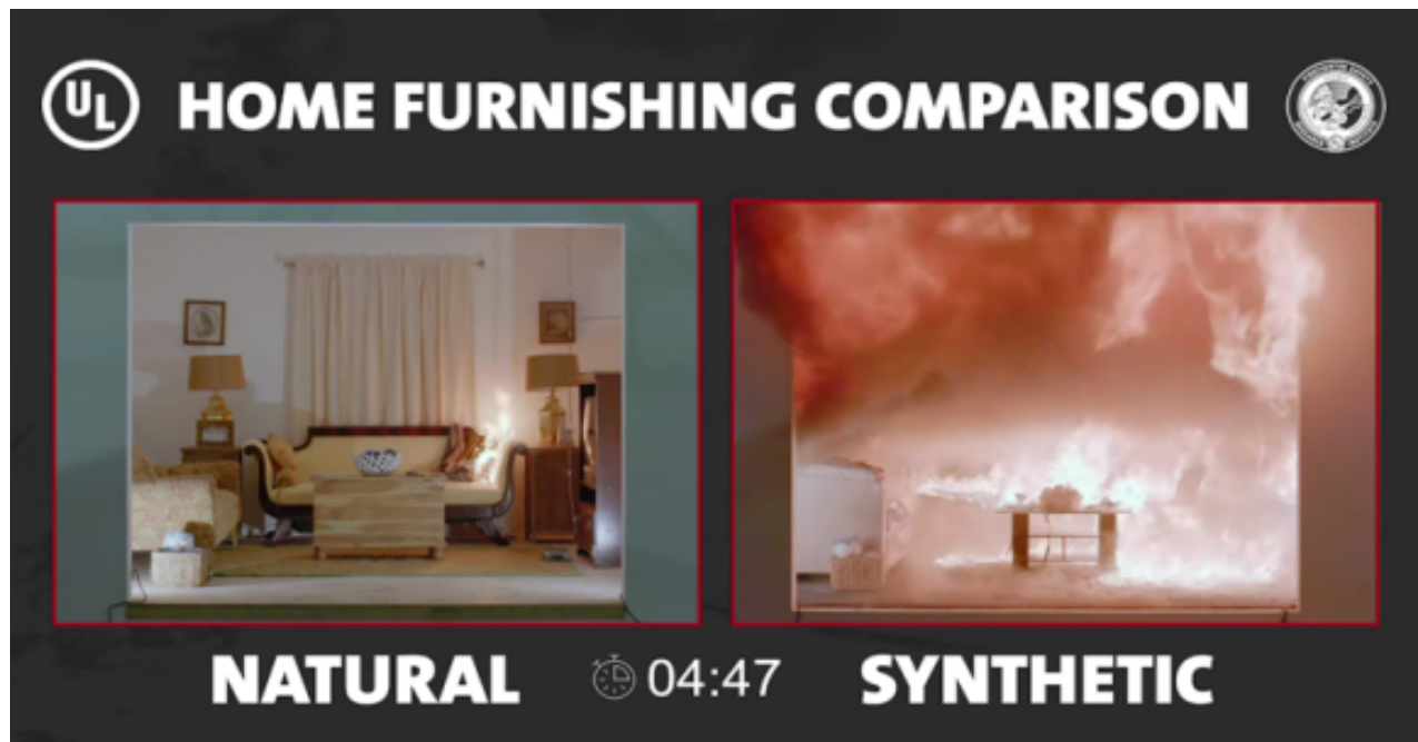
(Figure 1) Screenshot of UL FSRI Home Furnishings Comparison (Natural vs. Synthetic) video showing the difference in fire growth rate and flashover times due to the change in contents.
