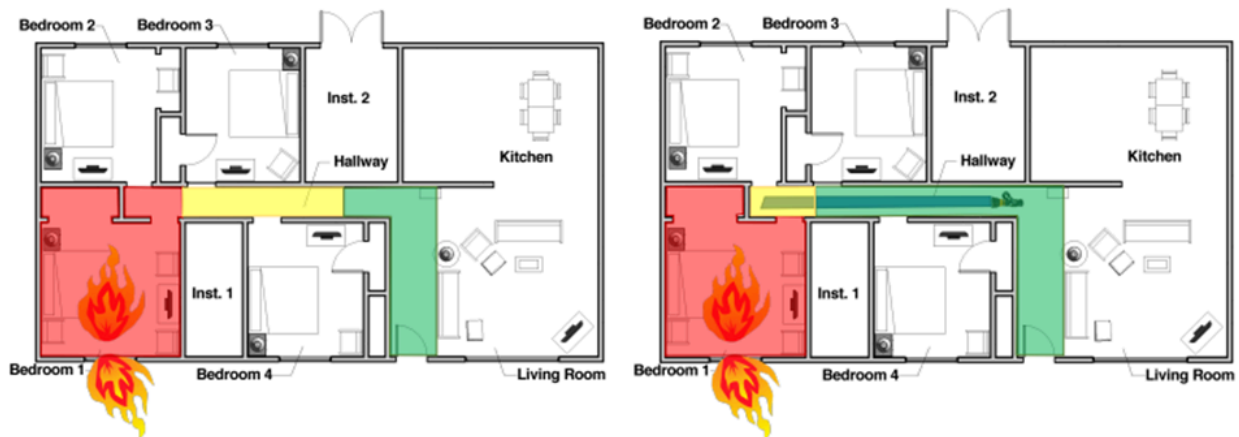
(Figure 5) Thermal conditions before (left) and after (right) water application down the hallway during an interior suppression tactic in Experiment 7. Color conditions represent operating zones where green is routine, yellow is ordinary, and red is emergency. This figure is from FSRI’s Impact of Fire Attack Utilizing Interior and Exterior Streams on Firefighter Safety and Occupant Survival: Full-Scale Experiments technical report (p. 181).
